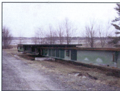
Fig. 2: Salvaged bridge steel at one of NEPCOAT's overcoating test sites
